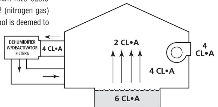
Figure 3 - Outdoor air and chlorine removal filters significantly change equilibrium point for highest ratio.
